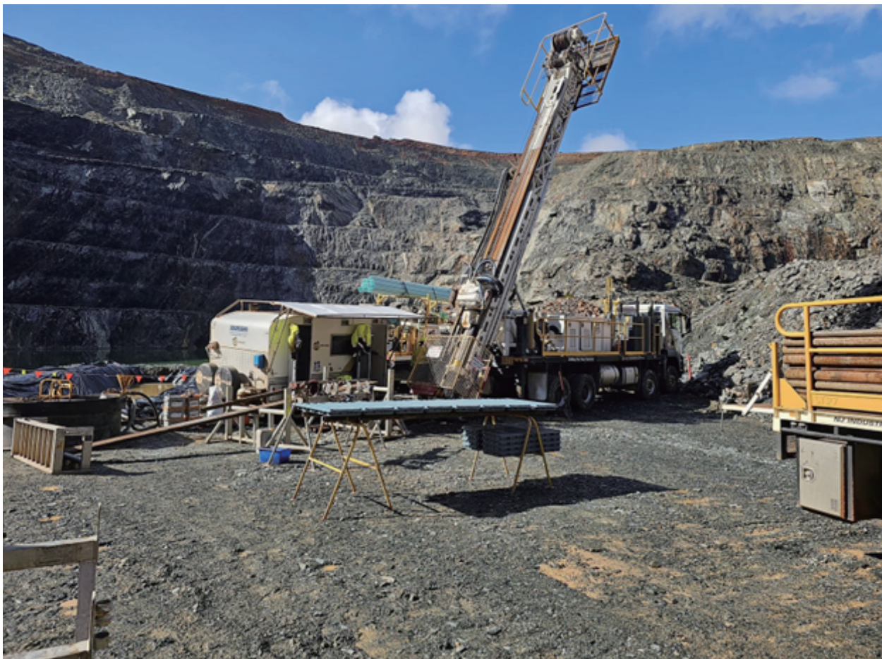
Figure 6, diamond drilling program commenced at Copperhead for the purpose of geotechnical investigation.
