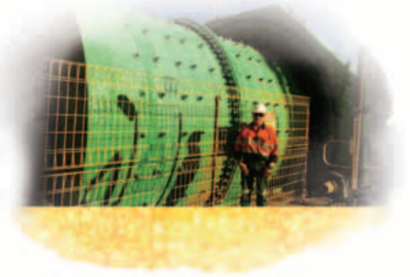
Photo of refurbished ball mill at the Marvel Loch Processing Plant
