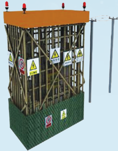
Protection for transformer
