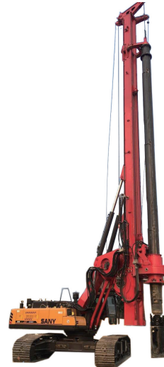
Rotary drilling rig
