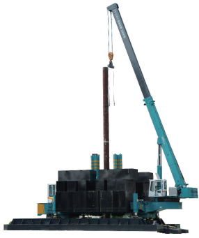
Static hydraulic pile machine
