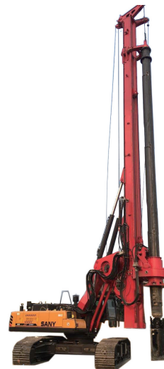
Rotary drilling rig
