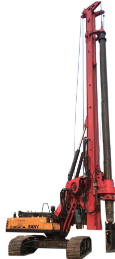
Rotary drilling rig
