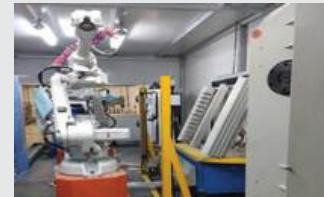
Automatic robotic arms for polishing process
