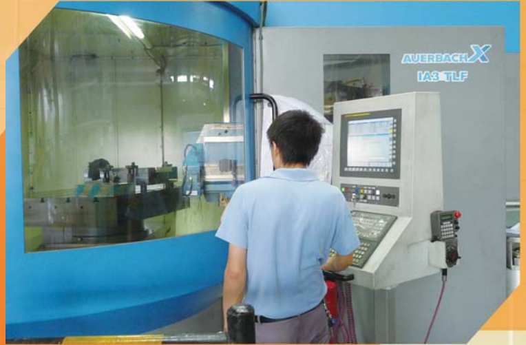
精密五軸深孔加工中心正在進行模架運水孔加工 Coolant hole drilling of a mould base on a precision 5-axis deep hole drilling center
