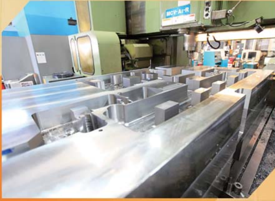
大型精密龍門式加工中心正在加工一件汽車配件模板 Machining of a mould plate for an automotive mould on a high precision double column machining center
