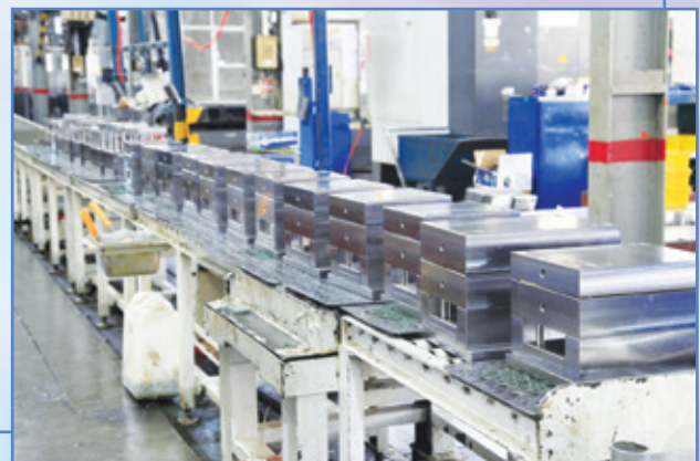
正在組裝的標準模架 Standard mould bases are being assembled
